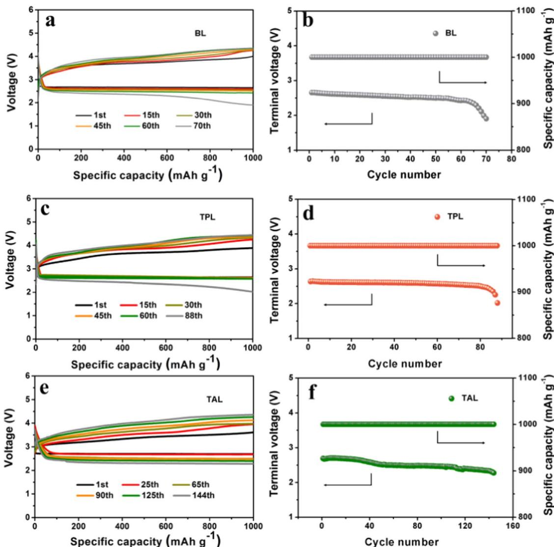
**Fig. 3.** Discharge-charge curves of Li-O<sub>2</sub> batteries with a) BL, c) TPL, and e) TAL anode and the corresponding terminal voltage curves with b) BL, d) TPL, f) TAL. All battery performances shown in this figure were tested with a fixed capacity of 1000 mA h g<sup>-1</sup> at a current density of 300 mA g<sup>-1</sup>.
