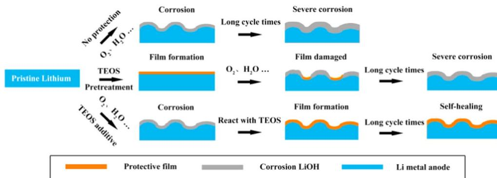
**Fig. 6.** The protection mechanism comparison of the three kinds of lithium metal anodes.
