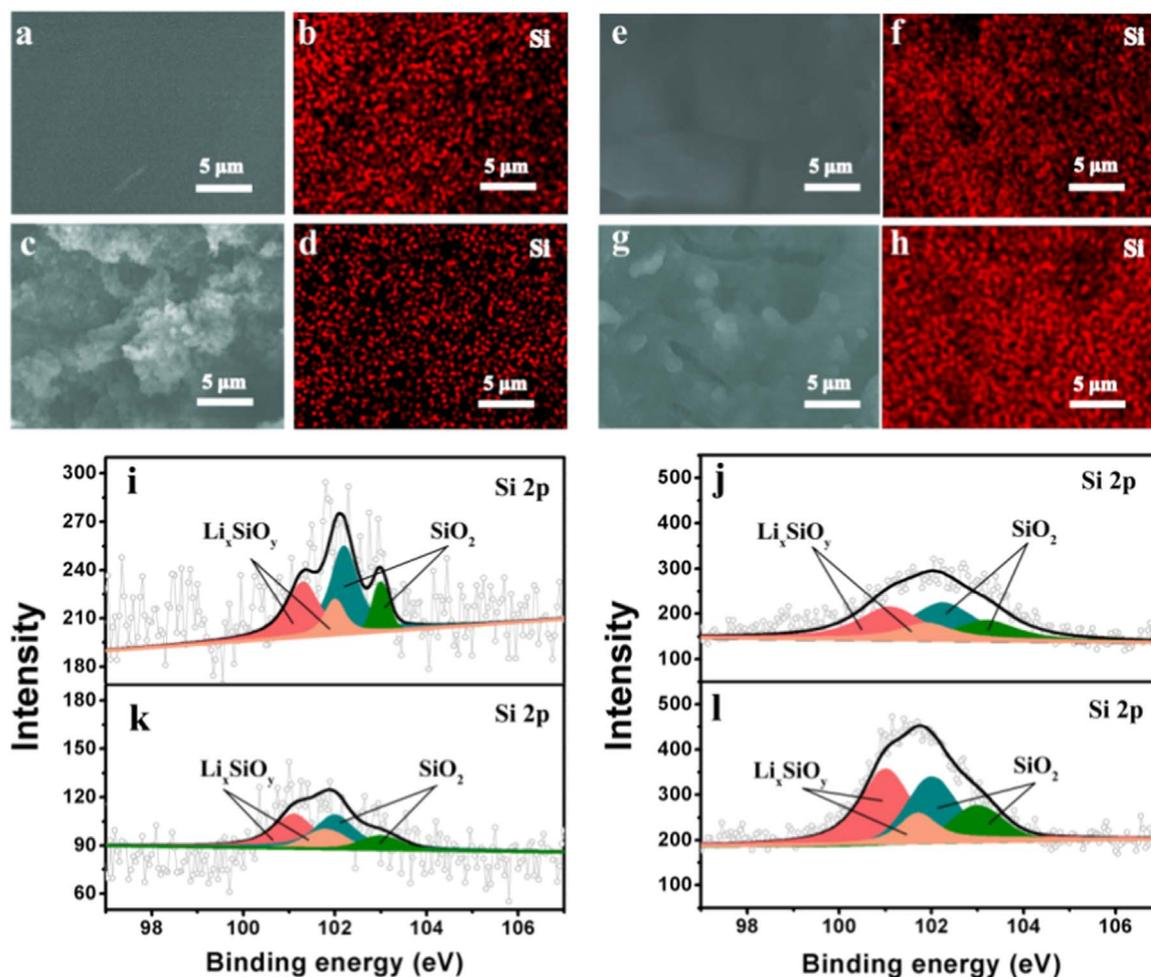
**Fig. 5.** a) SEM images of TPL and b) corresponding Si element mapping of TPL before cycling, c) SEM images of TPL and d) corresponding Si element mapping of TPL after 50 cycles. e) SEM images of TAL and f) corresponding Si element mapping of TAL after one cycle, g) SEM images of TAL and h) corresponding Si element mapping of TAL after 50 cycles. Si 2p XPS spectra of TPL i) before cycling, k) after 50 cycles. Si 2p XPS spectra of TAL j) after one cycle, l) after 50 cycles.
