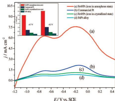
**Figure 2.** Comparison of catalytic activities for AB oxidation of (a) carbon-supported Fe@Pt NPs with amorphous iron cores, (b) commercial Pt, (c) Fe@Pt NPs with crystallized iron cores, and (d) the FePt alloy. Electrolyte: 0.01 M  $\text{NH}_3\text{BH}_3$ /1 M NaOH; sweep rate: 10  $\text{mV s}^{-1}$ ; rotation rate: 1600 rpm; room temperature; Pt loading: 24.6  $\mu\text{g cm}^{-2}$ . Inset: Comparison of the mass activities at  $-0.7$  and  $-0.2$  V.
