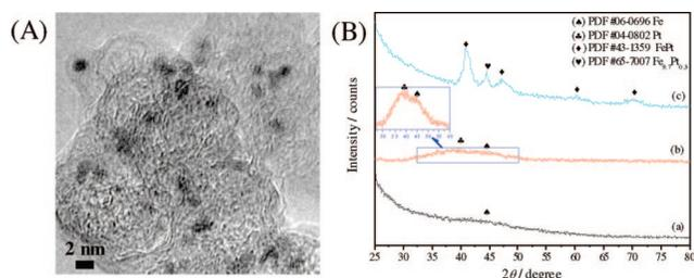
**Figure 1.** (A) TEM image of carbon-supported Fe@Pt NPs and (B) XRD patterns of (a) Fe cores reduced by NaBH<sub>4</sub> and NH<sub>3</sub>BH<sub>3</sub> before Pt replacement, (b) Fe@Pt NPs, and (c) Fe@Pt NPs after heat treatment at 823 K for 3 h under an argon atmosphere.
