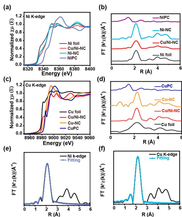
**Figure 2.** Structural characterization. (a, b) XANES spectra of Ni K-edge and FTs of  $k^3$ -weighted Ni K-edge EXAFS data for Cu/Ni–NC, Ni–NC, NiPC and Ni foil. (c, d) XANES spectra of Cu K-edge and FTs of  $k^3$ -weighted Cu K-edge EXAFS for Cu/Ni–NC, Cu–NC, CuPC and Cu foil. (d, e, f) Experimental and the fitting Ni and Cu K-edge EXAFS curves in R space of Cu/Ni–NC.
