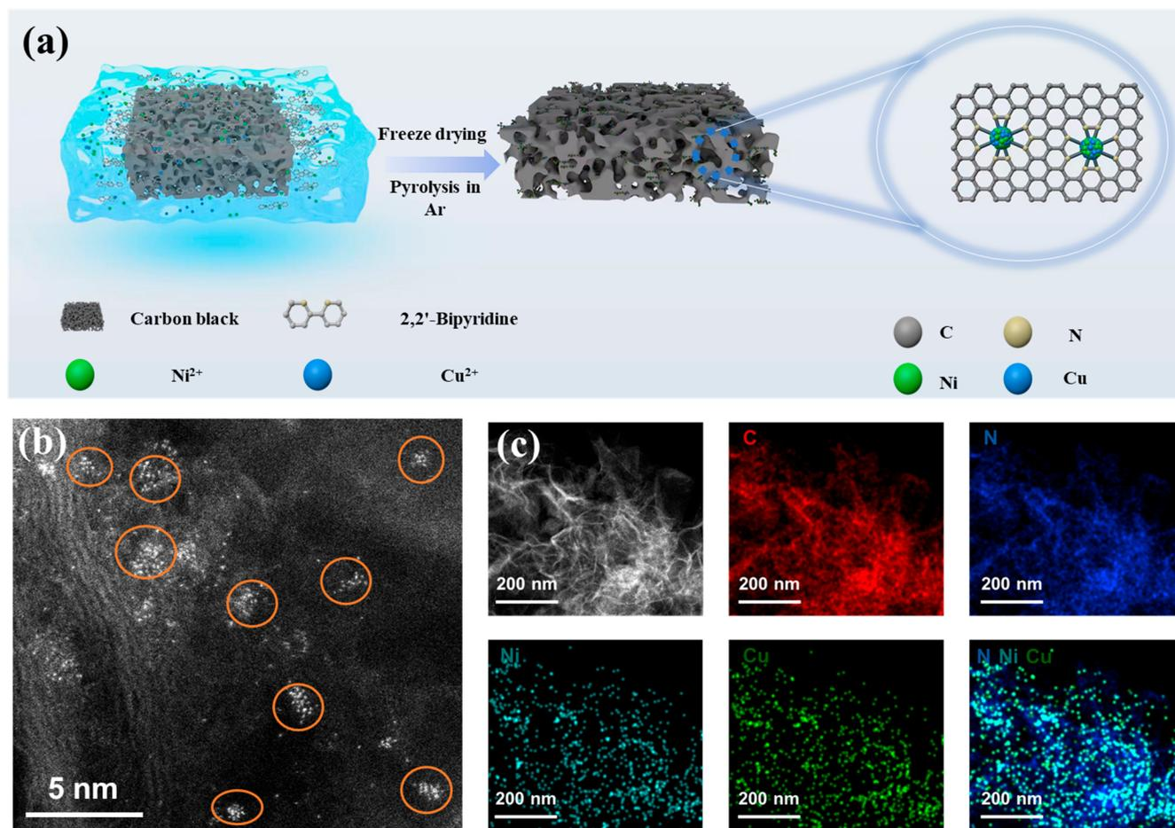
**Figure 1.** Synthesis and morphology characterization. (a) Schematic illustration of Cu/Ni-NC synthesis. (b) HAADF-STEM image of Cu/Ni-NC. (c) EDS (energy dispersive spectrometer) mappings of C, N, Cu and Ni elements of Cu/Ni-NC.
