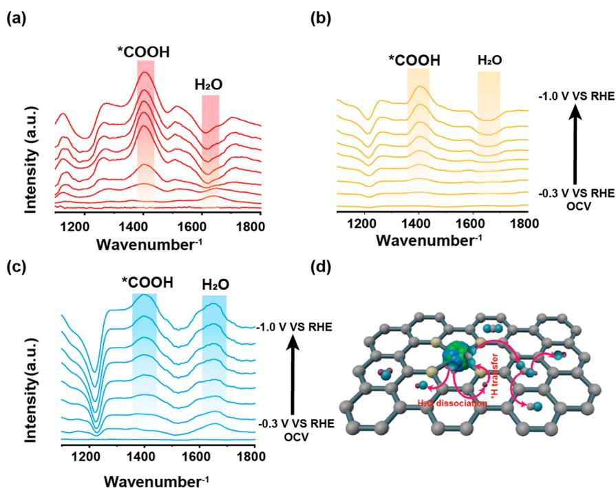
**Figure 5.** In situ ATR-SEIRAS recorded during ECO<sub>2</sub>R (a) Cu/Ni-NC. (b) Cu-NC. (c) Ni-NC. (d) Proposed catalytic mechanism of Cu/Ni-NC for ECO<sub>2</sub>R.
