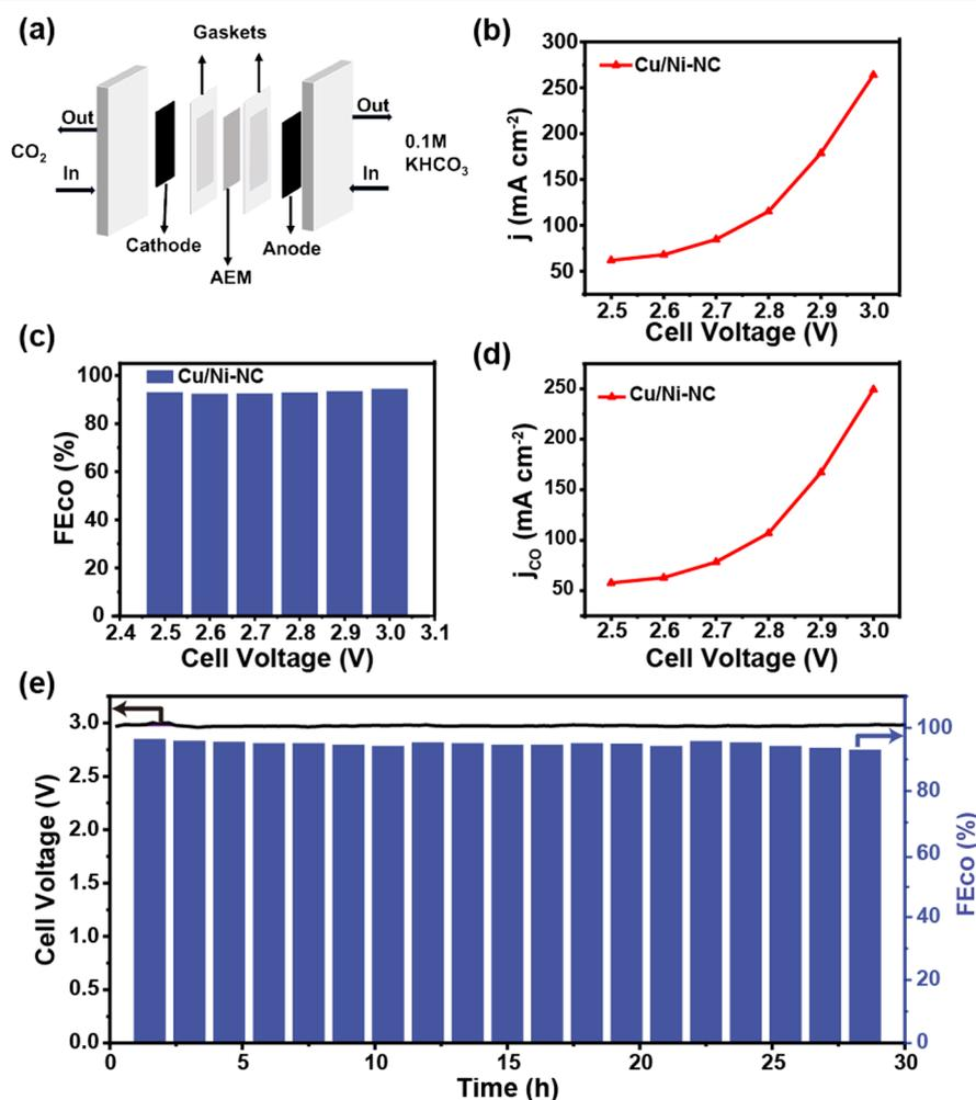
**Figure 4.** Electrochemical performance tested in a MEA electrolyzer. (a) Schematic illustration of the electrolysis device. (b)  $j$  of Cu/Ni-NC under different cell voltages. (c)  $\text{FE}_{\text{CO}}$  of Cu/Ni-NC under different cell voltages. (d)  $j_{\text{CO}}$  of Cu/Ni-NC under different cell voltages. (e) Stability of Cu/Ni-NC electrode under  $200$   $\text{mA cm}^{-2}$ .
