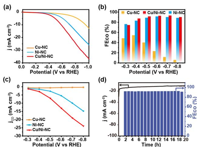
**Figure 3.** Electrochemical performance tested in H-cell. (a, b) LSV curves obtained in  $\text{CO}_2$ -saturated electrolyte (0.5 M  $\text{KHCO}_3$ ) and  $\text{FE}_{\text{CO}}$  over different potentials of the as-fabricated Cu/Ni-NC, Ni-NC and Cu-NC. (c)  $j_{\text{CO}}$  of the as-fabricated samples under different potentials. (d)  $j$  and  $\text{FE}_{\text{CO}}$  vs the electrolysis time for Cu/Ni-NC electrode under  $-0.7$  V vs RHE.
