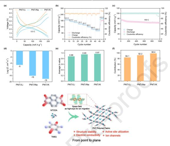
An iterative design process of polymer fabric from point to line and plane, inspired by the fabric craft, has been rationally designed to improve the electrochemical performance of organic electrode materials (OEMs) in rechargeable metalorganic batteries (MOBs). The evolution from point to line and plane of OEM improves its structure stability, kinetics, and utilization of active sites, benefitting the construction of high-performance MOBs.
